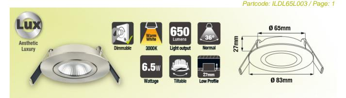
The Lux Ultra Slim high-end tiltable and dimmable downlight range impresses by offering stylish high-quality finish, ultra-low profile height of only 27mm, a modern look topped with a very efficient performance. A tiltable angle of up to 25 Degrees is ideal for directing light on to features or placement into a sloped ceiling.
